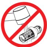
Do not rinse the EZ-Clean Membrane™ horizontally under running water – doing so may destroy the hollow fibers
